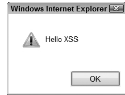
FIGURE 3-2: An example of a simple XSS attack
