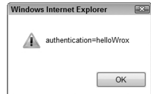
FIGURE 3-3: An example of an XSS-created alert box containing a site’s cookies
